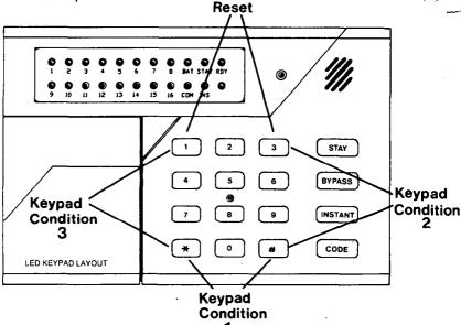
The keypad emergency conditions are programmable and can be used for conditions such as PANIC, FIRE, or MEDICAL Emergency. These conditions can be programmed by your installer to suit your needs. The keypad emergency conditions are active 24 hours a day, whether the system is armed or disarmed.
