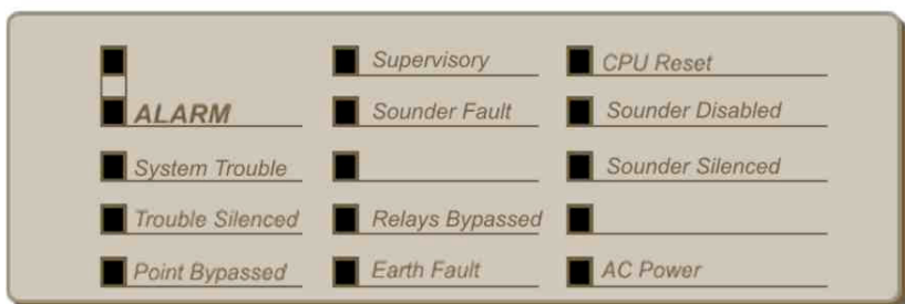
Figure 4: System Control LED Display
